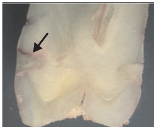
Figure 3: Grade II Dye Penetration more than half of cavity depth.
