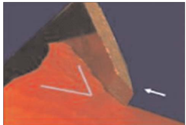
Figure 5b: Negative Rake Angle (Acute Angle)
