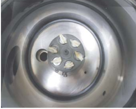
Figure 2 : Teeth Samples Mounted For Gold Sputtering
