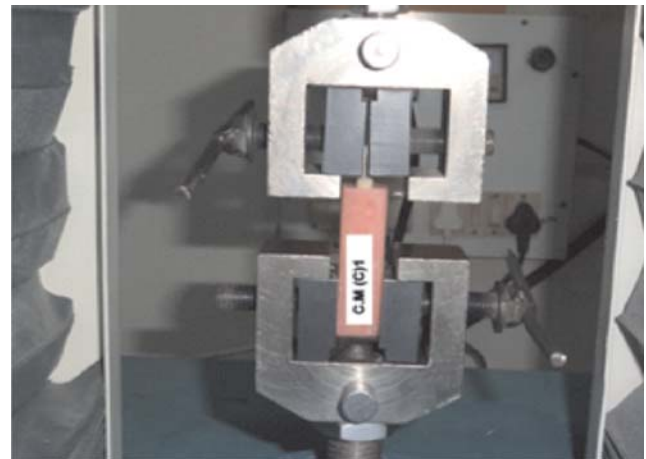
Figure 4: Universal testing machine for testing retentive strength
