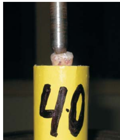
Figure 6: Steel bar touching cuspal inclines during fracture resistance test
