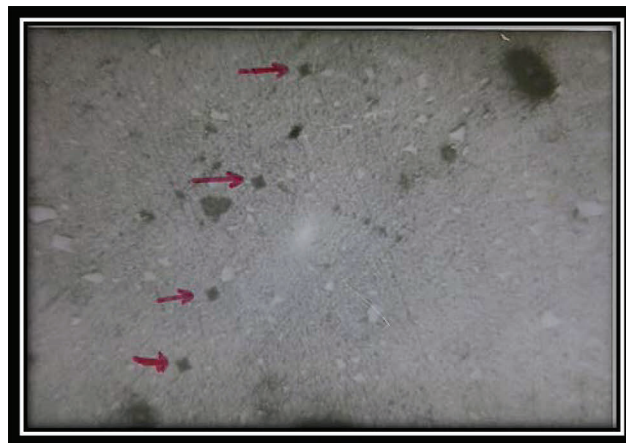
Fig. 4 Indentations obtained on resin surface (see red arrow) at \times 100 .
